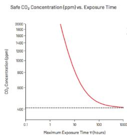
For an exposure time of  hours, the calculated safe time-averaged CO<sub>2</sub> concentration in this space is **928 ppm**.
