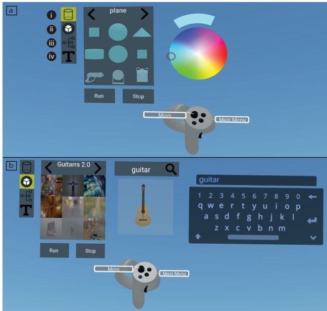
Figure 2: The palette menu of FlowMatic. (a)/(i) is the interface that allows users to import primitive models and select their colors using the color palette. (b)/(ii) is the interface that allows users to browse, search for, and import models from online. (iii) is a toggle for displaying the FRP diagram. (iv) allows users to create text elements in the scene.
