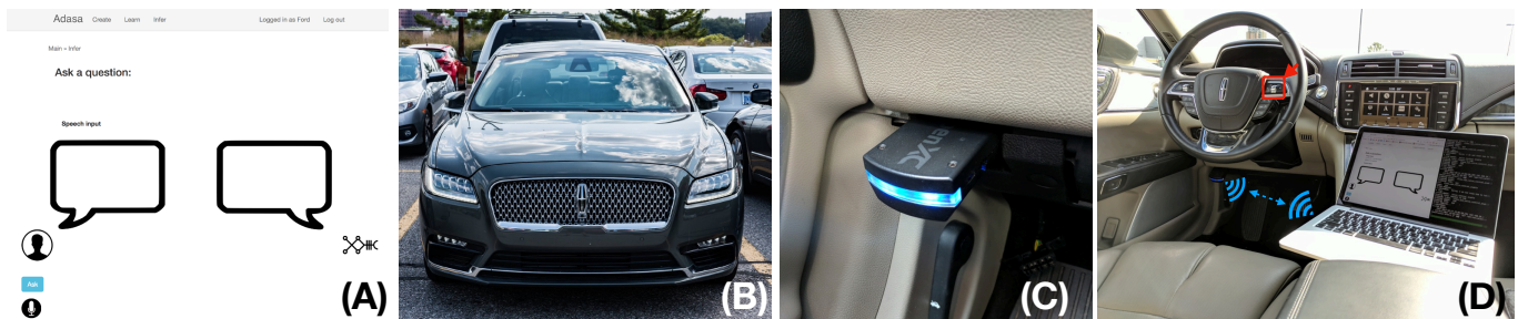
Figure 1: (A) The proposed digital assistant, Adasa, identifies user's questions or commands regarding ADAS features in human language and responds with answers or actions accordingly. (B) Adasa is integrated into a commercially available vehicle for evaluation and a real-world driving user study. (C) Adasa is able to access vehicle CAN signals via Bluetooth to conduct system diagnosis or system control. (D) Adasa setup, driver enables Adasa by pressing the button on the wheel to start the conversation.
